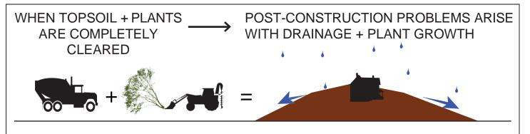
The use of heavy construction vehicles, combined with the clearing of most trees, shrubs, and topsoil, leaves homeowners with damaged, compacted soil and future problems.
