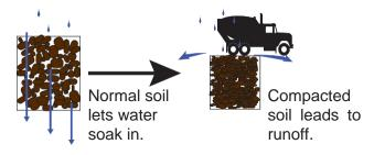
Driving + parking heavy equipment on your property without careful planning will damage soil, limiting water infiltration and creating future stormwater management problems.
