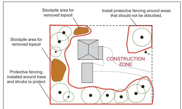
Make a map showing how you want to limit the construction footprint. Work with your contractor to clarify where you will put protective fencing and stockpile topsoil for later use.
